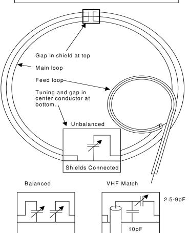
Coax feed loop is approx. 1/3 the dia. of the main loop. Strip ½" of outer jacket and shield/braid from the end of the coax being careful not to cut through the dielectric.
